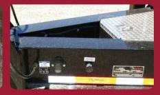
Conveniently located, easy to use controls for raising and lowering trailer and ramps.
