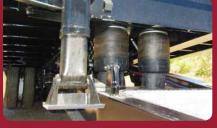
Pneumatically operated tilting deck and ramp design.
