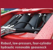
maximizes lift capacity and load height.
